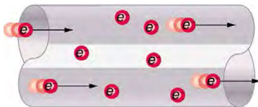
Figure 20.5 When charged particles are forced into this volume of a conductor, an equal number are quickly forced to leave. The repulsion between like charges makes it difficult to increase the number of charges in a volume. Thus, as one charge enters, another leaves almost immediately, carrying the signal rapidly forward.
