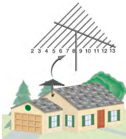
Figure 24.28 A television reception antenna has cross wires of various lengths to most efficiently receive different wavelengths.
