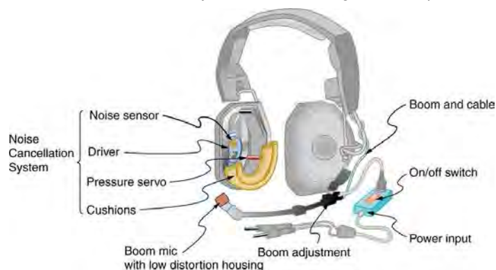
Figure 17.23 Headphones designed to cancel noise with destructive interference create a sound wave exactly opposite to the incoming sound. These headphones can be more effective than the simple passive attenuation used in most ear protection. Such headphones were used on the record-setting, around the world nonstop flight of the Voyager aircraft to protect the pilots' hearing from engine noise.
