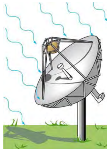
Figure 24.29 Satellite dishes receive TV signals sent from orbit. Although the signals are quite weak, the receiver can detect them by being tuned to resonate at their frequency.
