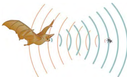
Figure 17.11 A bat uses sound echoes to find its way about and to catch prey. The time for the echo to return is directly proportional to the distance.
