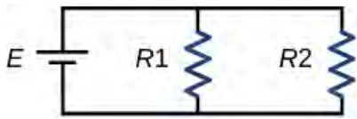
Figure 21.68 In an experiment this circuit is set up. Three ammeters are used to record the currents in the three vertical branches (with R_1 , R_2 , and E ). The readings of the ammeters in the resistor branches (i.e. currents in R_1 and R_2 ) are 2 A and 3 A respectively.
