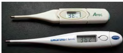
Figure 20.15 These familiar thermometers are based on the automated measurement of a thermistor's temperature-dependent resistance. (credit: Biol, Wikimedia Commons)
