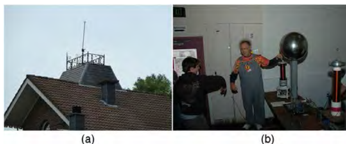
Figure 18.25 (a) A lightning rod is pointed to facilitate the transfer of charge. (credit: Romaine, Wikimedia Commons) (b) This Van de Graaff generator has a smooth surface with a large radius of curvature to prevent the transfer of charge and allow a large voltage to be generated. The mutual repulsion of like charges is evident in the person's hair while touching the metal sphere. (credit: Jon 'ShakataGaNai' Davis/Wikimedia Commons).
