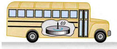
Figure 10.16 Experimental vehicles, such as this bus, have been constructed in which rotational kinetic energy is stored in a large flywheel. When the bus goes down a hill, its transmission converts its gravitational potential energy into KE_{\text{rot}} . It can also convert translational kinetic energy, when the bus stops, into KE_{\text{rot}} . The flywheel's energy can then be used to accelerate, to go up another hill, or to keep the bus from going against friction.
